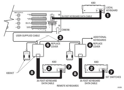
Figure 1. Wiring Diagram for Local/Remote Keyboards
